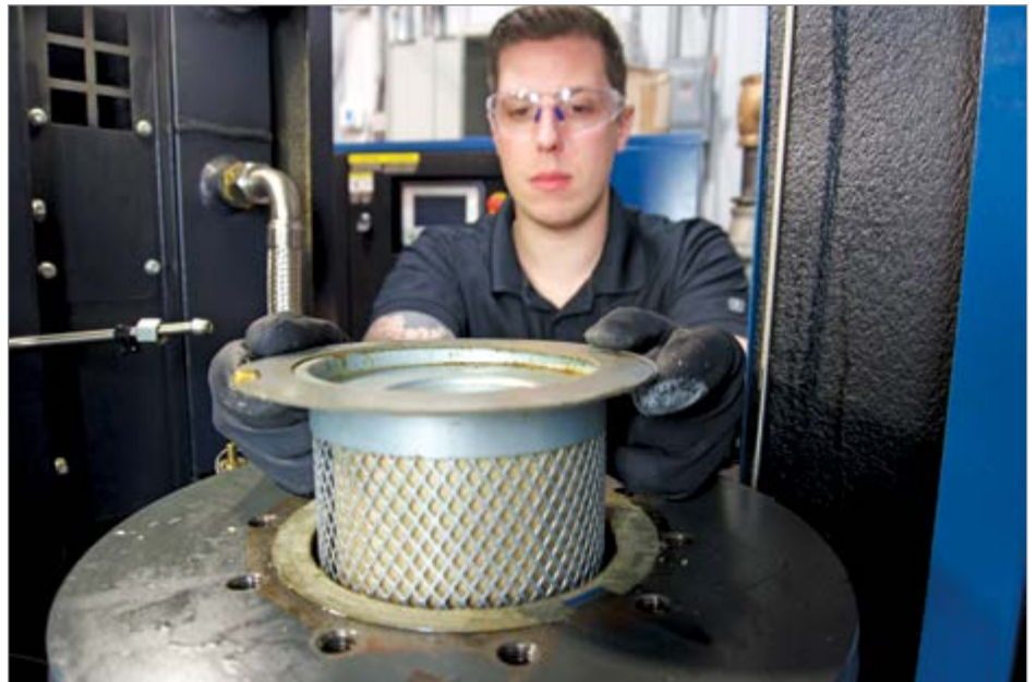
To keep oil carryover below the manufacturer's three parts per million, follow a preventive maintenance program: Check the air-oil separator annually and replace inline filters every six months.
