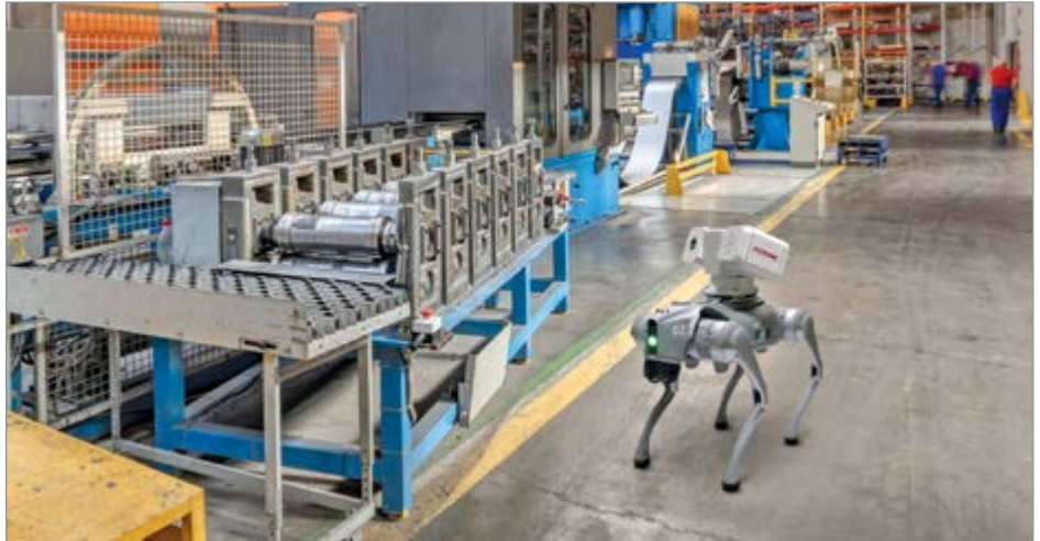
FOTRIC TD2 sense Acoustic Imaging Module monitoring a manufacturing facility, detecting leaks and operational anomalies.
